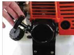
5. After the engine has started, slide the choke knob down slowly to the opened position
